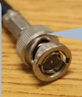
**BNC** - A professional type of video connector featuring a two-pin lock. Audio is not carried by this connection.
