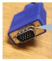
**VGA** - Video Graphics Array, a high quality analog connection used primarily for computer video connections.
