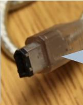
Firewire -Firewire (also called IEEE1394 High Performance Serial Bus) is a technology for high-speed data transfer over a cable. It is often used for connecting digital video cameras or hard drives to computers.
