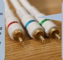
**Component** - This high quality option is the minimum standard for high definition video. It can used by hi-def cable and satellite providers as well as DVD and Blu-ray Disc players. It requires three cables (blue, red, green). Audio is not carried by this connection.
