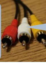
**Composite** - Cable for consumer analog TV signals from source to source or source to display. This connection gives the lowest video connection available. A yellow RCA Connector is typically used for composite video.
